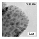
Ethene hydrogenation catalyzed by narrowly size-distributed Pd catalysts, produced by CVD, was investigated. A pronounced size dependence of TOF was found with a maximum at 3-4 nm.
